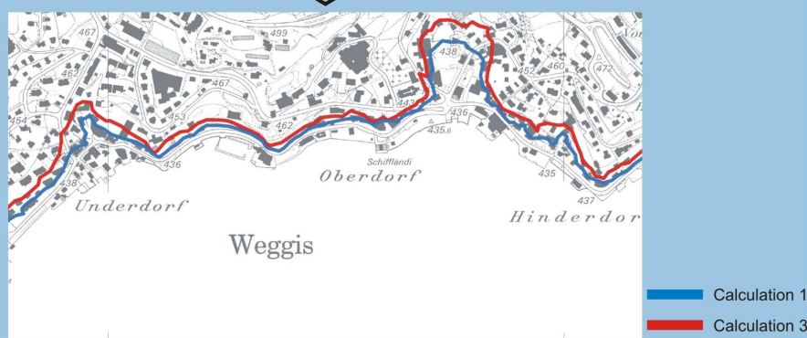
Fig. 6 Mapdetail showing the areas with a wave overtopping impact for calculation 1 and 3.
